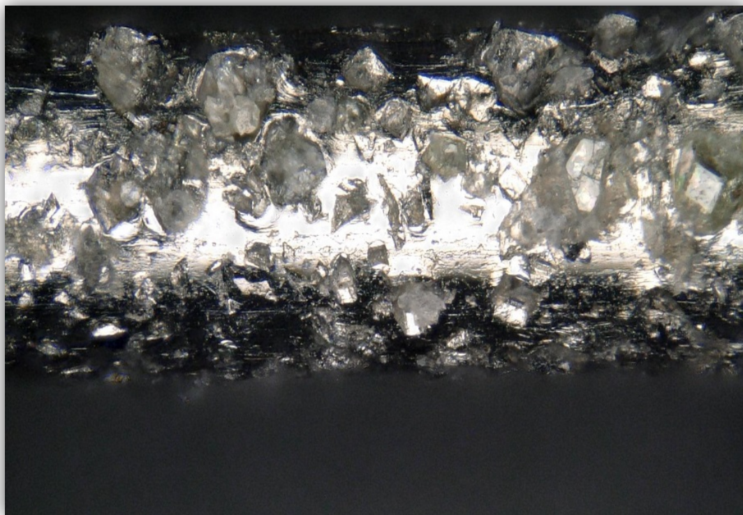
Well diamond wire: diamond grains embedded in the stainless steel wire support
