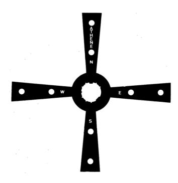
This consists of an inner ring of 4mm diameter (outside) and 2mm inside diameter. It has four arms each extending 6mm outwards.
