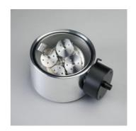
The motorised specimen stage with manual tilt delivered standard with the system has four holders which move in a non-repetitive rotary planetary motion. A choice of 4 speeds are available and the specimen platform can be tilted from 0-90°.
